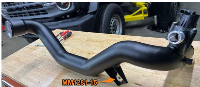
**15.** Using the provided clamps and turbo boot, install the Mishimoto hot-side intercooler pipe. Do not tighten the clamps, this will be done later. Reconnect the bypass valve hose and electrical harness.
