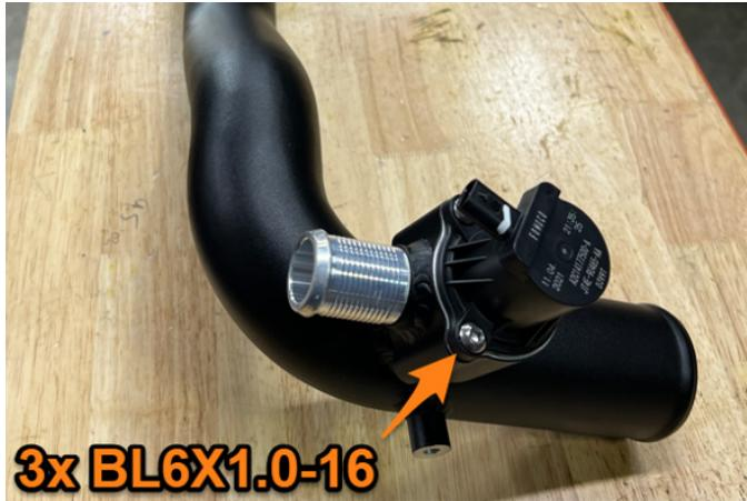
**14.** Install the provided grommet to the Mishimoto hot-side intercooler pipe. (MM1281-15)
