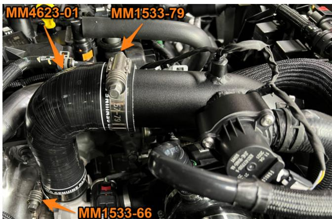
**16.** Secure the Mishimoto hot-side intercooler pipe to the bracket on the front of the engine using the provided hardware. (Flange-Head M6X1.0-30)
