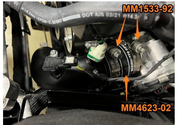
**19.** Install the Mishimoto intercooler and reinstall the lower intercooler mounting brackets.
