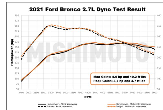
**Figure 15:** The Mishimoto intercooler yielded a max gain of 8.0 hp and 10.2 ft-lbs of torque.
