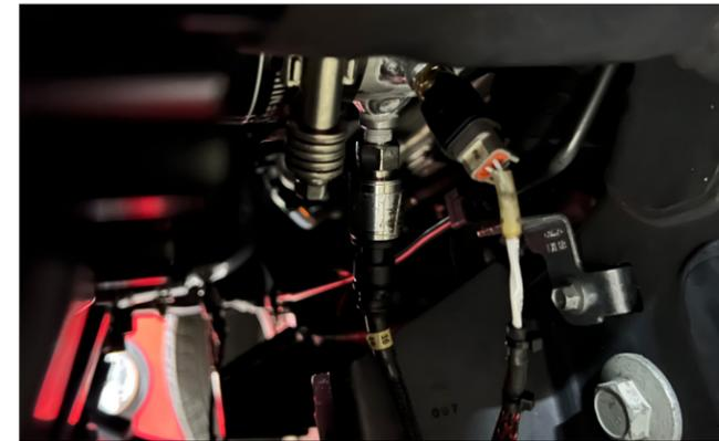
**Figure 5:** Pressure and temperature sensors installed in the cold-side intercooler piping.
