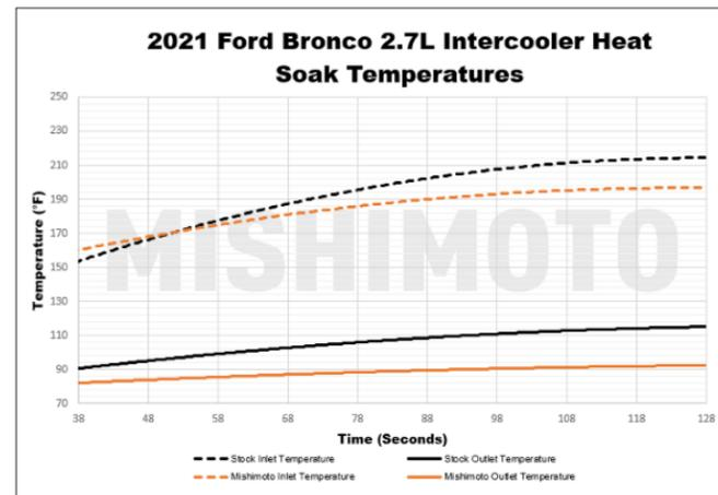
**Figure 11:** The Mishimoto intercooler reduced outlet air temps. by 15.5°F (8.8°C) on the 2.7L Bronco.
