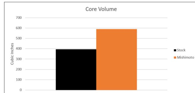
**Figure 1:** The Mishimoto intercooler has a 49% increase in overall core volume compared to the stock intercooler.
