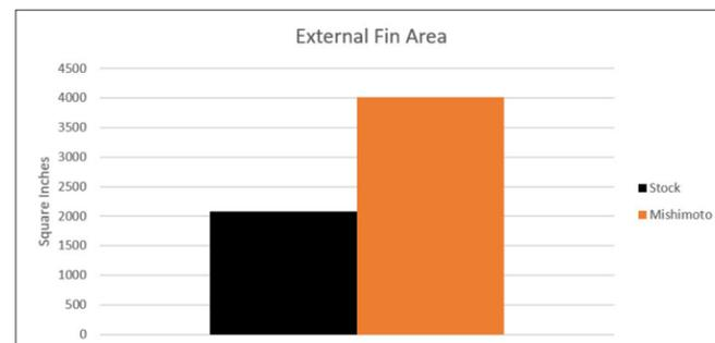
**Figure 2:** The Mishimoto intercooler has a 93% increase in fin surface area over the stock intercooler.
