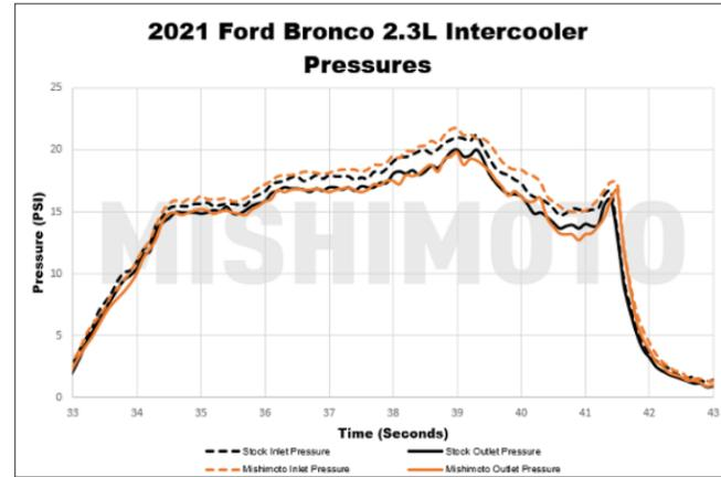
**Figure 12:** The Mishimoto intercooler had an additional 1.0 psi of boost pressure drop compared to the stock intercooler on the 2.3L Bronco.
