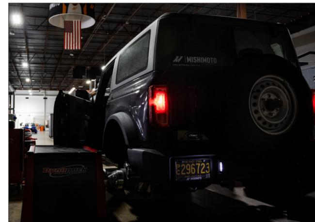
**Figure 6:** A Dynapack dynamometer was used for 2.3L testing.
