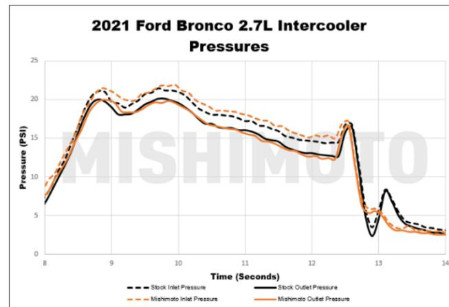
**Figure 13:** The Mishimoto intercooler had an additional 1.0 psi of boost pressure drop compared to the stock intercooler on the 2.7L Bronco.
