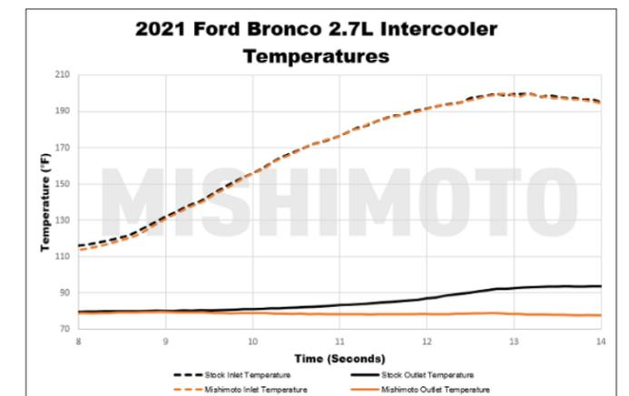
**Figure 9:** The Mishimoto intercooler reduced outlet air temps. by 15.5°F (8.8°C) on the 2.7L Bronco.
