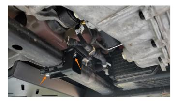
**03.** Using a 13mm socket, install the Borne Off-Road transfer case skid plate with the (4) bolts that were removed in step 1. Do not fully tighten the bolts yet.
