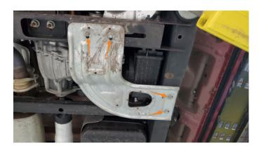
**02.** Using a 13mm socket, assemble the upper and lower brackets with (2) of the supplied bolts, flat washers, & lock washers around the frame as shown below. Leave the bolts loose enough that the location of the bracket on the frame can be adjusted.
