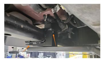
06. Using a 13mm socket, fully tighten all (5) mounting bolts to22 lb-ft (30 N-m). (See image first image on right)
