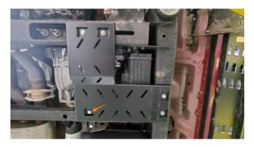
**05.** Using a 13mm socket or wrench, fully tighten the (2) bolts that assemble the bracket around the frame from step 2. Tighten to 22 lb-ft (30 N-m).
