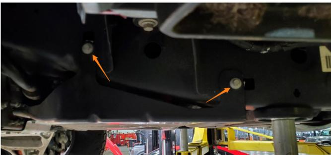
\*If an OEM splash guard is equipped (instead of a skid plate) remove the (2) bolts that attach the (2) brackets to the frame as well as the clip nuts. There is (1) on the driver side and (1) on the passenger side.
