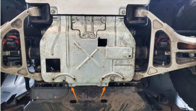
**03.** Using a 13mm socket, remove the transmission skid plate from the vehicle by removing the (4) bolts that attach it to the frame. There are (2) on the driver side and (2) on the passenger side.
