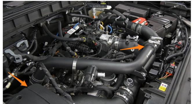
**30.** Adjust the pipes and boots until everything is aligned. The pipes are inserted far enough into the boots when the bead is roughly centered on the second white line from the edge of the boot. For cast/machined fittings, they should bottom out on the shoulder.
