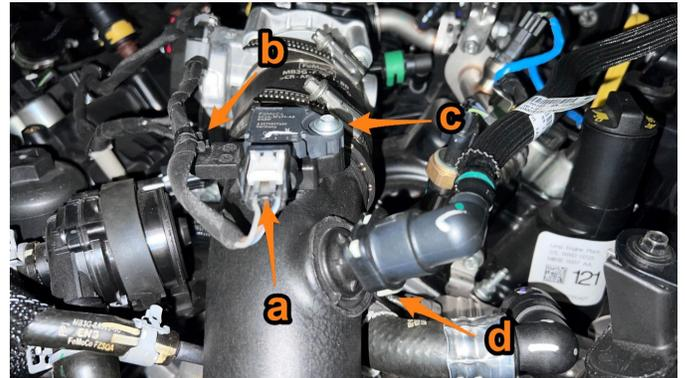
**7.** Using a 7mm socket, loosen hose clamps (a) and (b). Using an 8mm socket, remove bolt (c). Remove the intake pipe.
