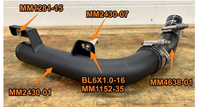
**24.** Install boot 2 onto hot-side pipe 2 then slide a 79mm clamp and 54mm clamp over the boot. Using a 3mm Allen wrench, install the 3 grub screws into the housing until they bottom out. Install the two grommets into the brackets.
