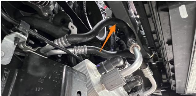
**14.** Using an 8mm socket, remove this bolt and tuck the hose/bracket out of the way.
