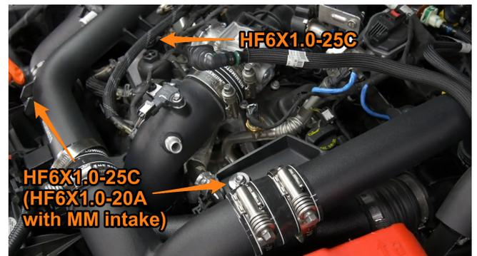
**32.** Using a 10mm socket, tighten all the hot-side pipe clamps. The clamp on the driver-side turbo outlet can be accessed through a hole in the fender liner.
