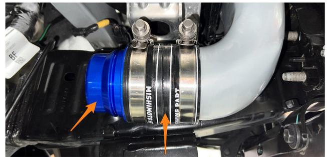
**18.** From the bottom of the vehicle, install cold-side pipe 1 on the passenger side and hot-side pipe 3 on the driver side. Reattach the ground strap from step 11.
