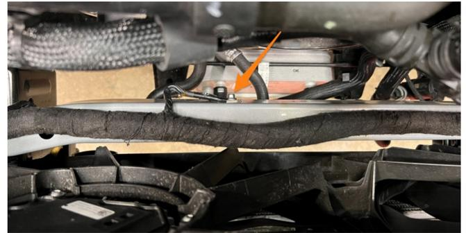
**12.** Using a 15mm socket, loosen the 2 rear bolts and completely remove the rest of the bolts. Remove the front skid plate/splash guard. Both the plastic splash guard and metal skid plate are shown below.
