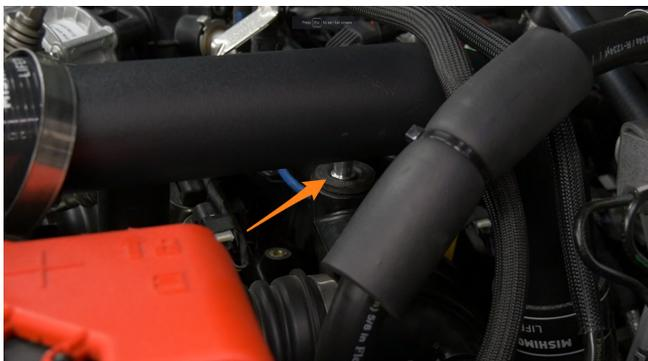
**28.** Install the lower boot of the assembly from step 26 onto the hot-side pipe coming from the intercooler, then slide the upper right boot onto the pipe from the previous step.
