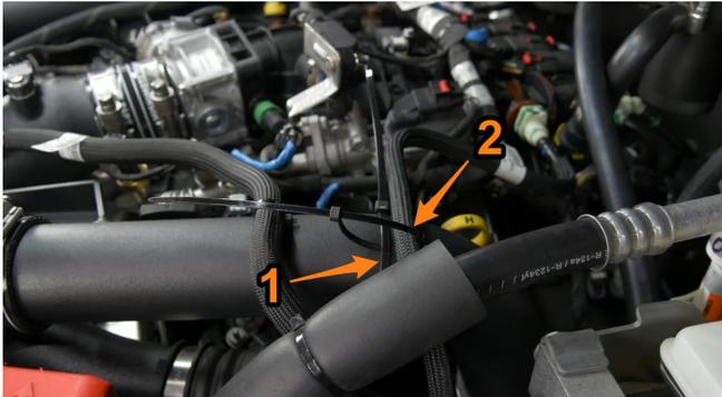
**35.** Rotate the hose/line from step 13 back into place and reinstall the bracket and bolt from step 14.
