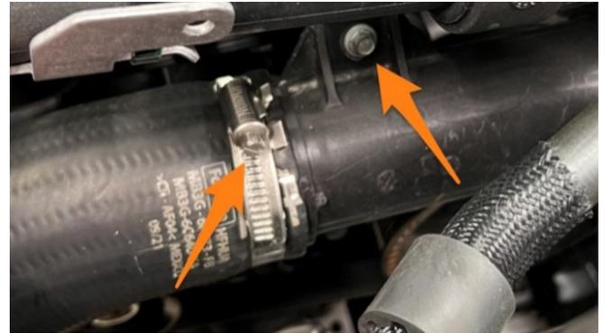
**11.** Using an 8mm socket, remove the bolt holding the ground strap and tuck the strap on top of the cross member.
