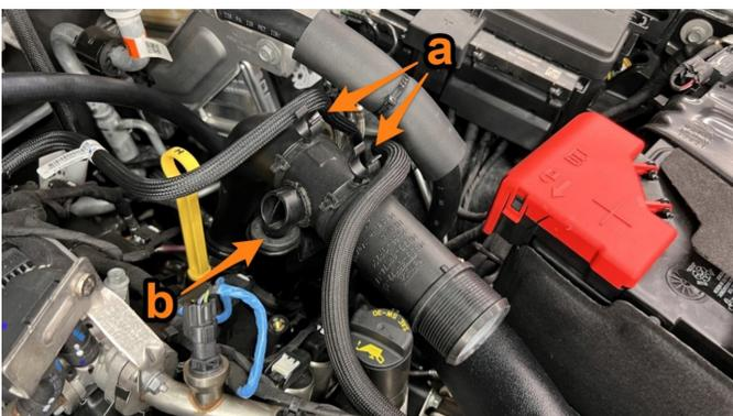
**6.** Unplug connector (a) and use a trim clip tool to remove tree clip (b). Using a T25 Torx, remove screw (c) and remove the sensor from the upper cold-side intercooler pipe.
