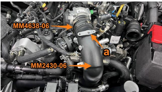
**22.** Reinstall the airbox and intake pipes.
