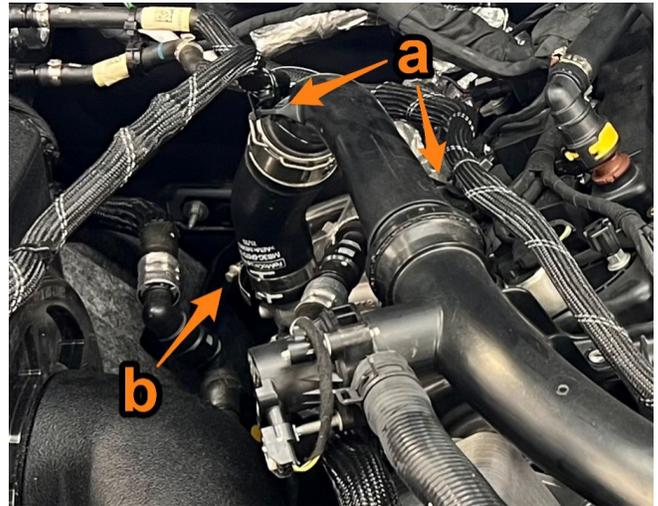
2. Unplug the recirculation valve connector (a) and remove the two wire clips (b). Disconnect the recirculation hose quick disconnect fitting from the air intake (c). Using an E5 Torx or 4mm socket, remove the 3 stud bolts and remove the valve from the stock intercooler pipe.
