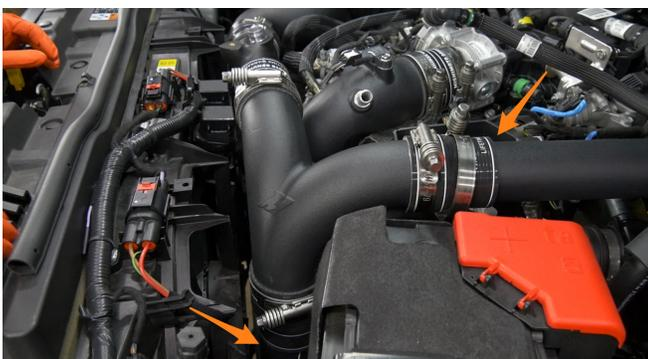
**29.** Install the assembly from steps 24/25 on the passenger-side of the engine, being sure to get the boot onto the turbo outlet and the other end of the pipe into the other side of the "Y" from the previous step.
