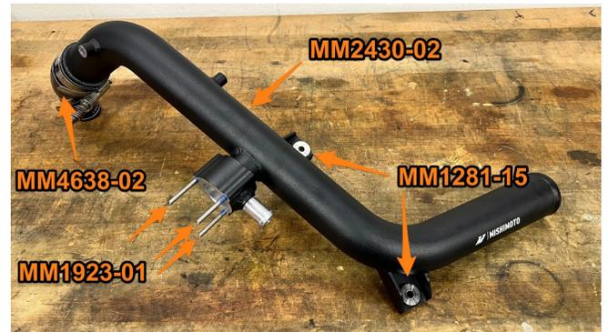
**25.** Using a 10mm socket, install the stock recirculation valve into the housing with the provided locking nuts.
