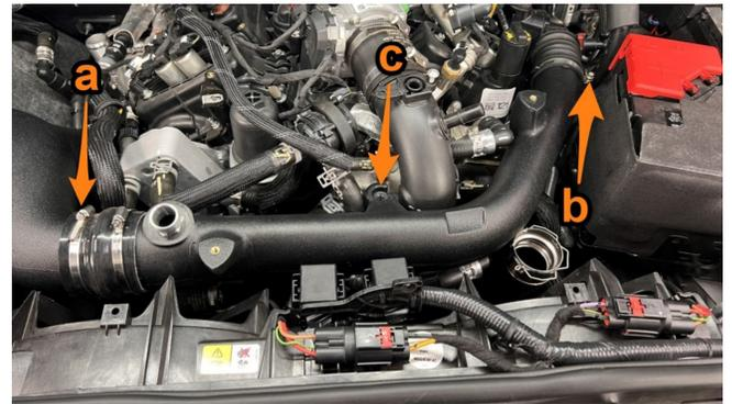
**8.** Using a 7mm socket, loosen the clamp on the passenger-side turbo.
