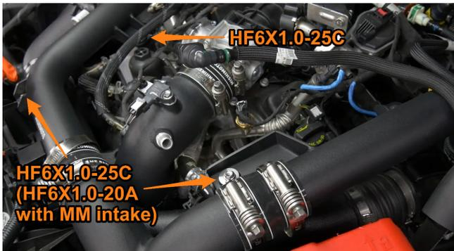
**33.** Using a 10mm socket, tighten all the hot-side pipe clamps. The clamp on the driver-side turbo outlet can be accessed through a hole in the fender liner.
