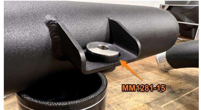
17. Swap the quick disconnect adapters on the Mishimoto stock-location Intercooler for the silicone boot adapters. Torque the bolts securing the adapters to the Intercooler to 10Nm [88.5 in-lbs].
