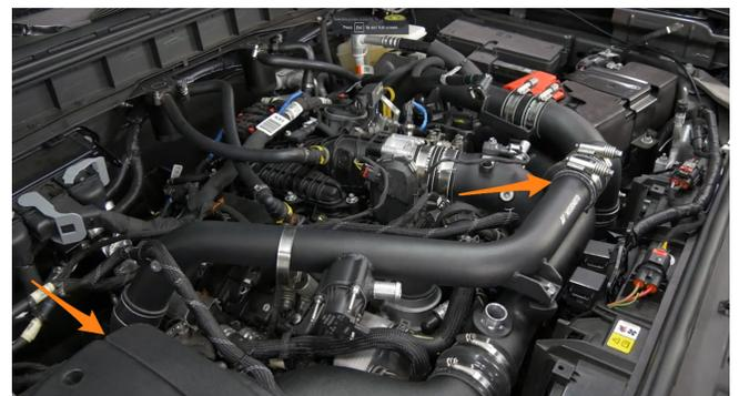
**31.** Adjust the pipes and boots until everything is aligned. The pipes are inserted far enough into the boots when the bead is roughly centered on the second white line from the edge of the boot. For cast/machined fittings, they should bottom out on the shoulder.
