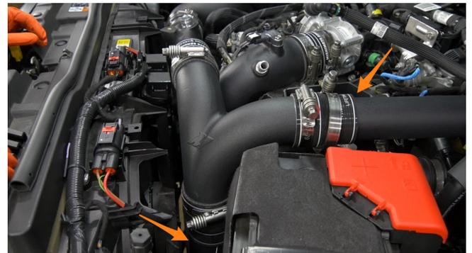
**30.** Install the assembly from steps 25/26 on the passenger-side of the engine, being sure to get the boot onto the turbo outlet and the other end of the pipe into the other side of the "Y" from the previous step.
