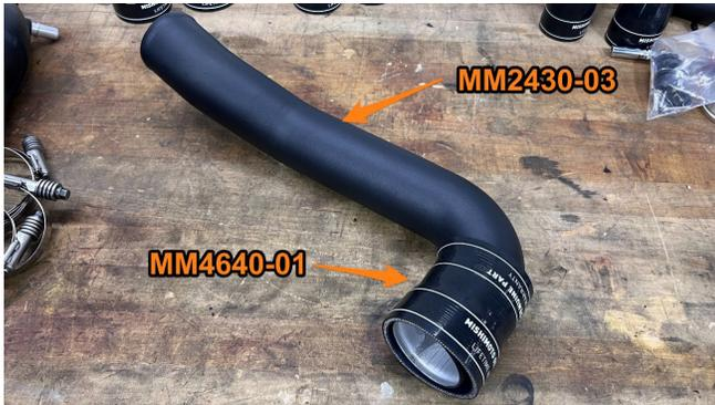
**19.** From the bottom of the vehicle, install cold-side pipe 1 on the passenger side and hot-side pipe 3 on the driver side. Reattach the ground strap from step 11.
