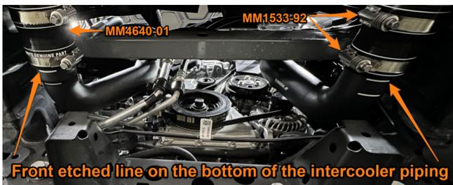
**21.** Using a 10mm socket and wrench, fasten the passenger-side Intercooler pipe to the bracket with the provided 6mm bolt and nut. Install the longer straight section of boot 5 onto the pipe and slide 2x 92mm clamps over the boot.
