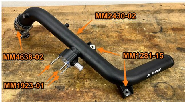
**26.** Using a 10mm socket, install the stock recirculation valve into the housing with the provided locking nuts.
