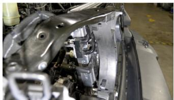
**8.** Secure the AC condenser mount to the radiator using the longest 10mm bolt in your kit. (1x HF6X1.0-30C)
