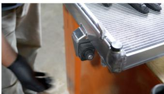
**3.** Separate the fan shroud from the stock radiator and install it to the Mishimoto radiator using the provided hardware.
