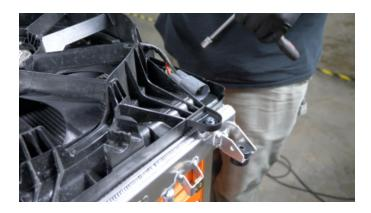
4. Lower the Mishimoto radiator and fan shroud into the engine bay.
