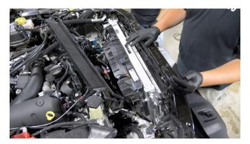
**5.** Reposition the transmission cooler and attach it to the radiator brackets.
