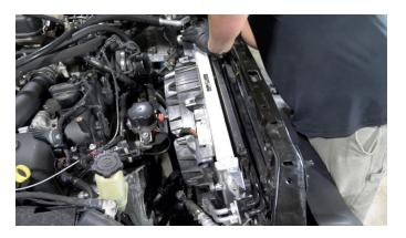
**6.** If installing on a 4-cylinder vehicle, secure the low-temp radiator, AC condenser, and battery radiator to the Mishimoto radiator using the provided hardware. [4x HF6X1.0-25B bolts] If installing on a 6-cylinder vehicle, secure the AC condenser to the Mishimoto radiator using the provided hardware.
