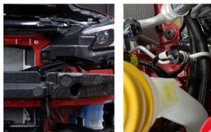
**17.** Install the oil lines onto the banjo bolts and then install the banjo bolts onto the sandwich plate. The shorter of the two lines goes to the passenger side of the sandwich plate and the longer line goes to the driver's side.
