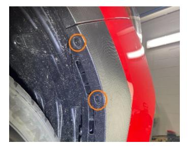
**06.** Remove the 5X pop clips, and 6X 10mm bolts at the top of the bumper and remove the black metal trim piece on top of the bumper.
