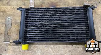
11. Prepare one of the included M8 bolts and install the oil cooler. Use the m8 bolt to hang the oil cooler from the factory hole (Bolt #1 in picture). Leave this bolt loose. Then, install the included M6 bolt through the core support and into the lower oil cooler bracket (bolt #2). Leave this bolt loose for now.
