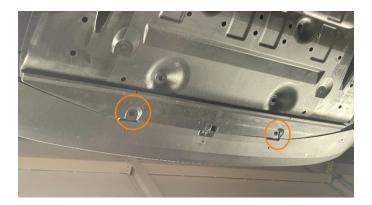
**05.** Remove the 2x pop clips for the bumper in each front wheel well (4x total) by pushing in the center until a click is heard. Then pull the pop clip out from the outer edge.
