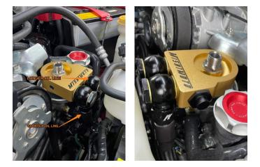
**19.** Fill the engine with oil if drained in step 2, then install the oil filter. Note: The oil filter will protrude past the sandwich plate, however, the seal will still be fully seated on the sandwich plate.
