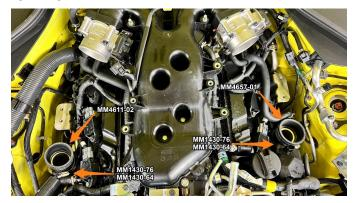
**21.** Install the intercoolers into the vehicle throttle body side first, followed by the turbo side. You can run a large pick between the turbo coupler and the intercooler snout while pushing down to help get the coupler over the intercooler barb.
