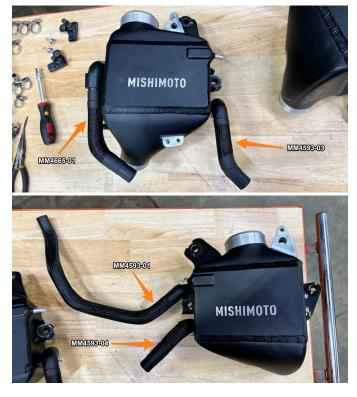
**19.** Install the two sensors removed in step 14 into the Mishimoto intercoolers using the stock bolts (10mm socket). Install a coupler onto each intercooler and slide two 65-89mm worm gear
