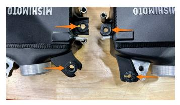
**17.** Install the brackets onto the intercoolers using the provided hardware (10mm socket). Install two of the stock grommets into each of the brackets as shown.
