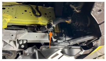
4. While waiting for the system to drain, use a 14mm socket to remove the four bolts and 2x nuts securing the strut bar. Then, remove the strut bar.
