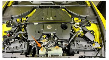
**3.** Place a suitable container below, and using a Phillips head screwdriver, remove the drain plug for the charged air cooling system.
