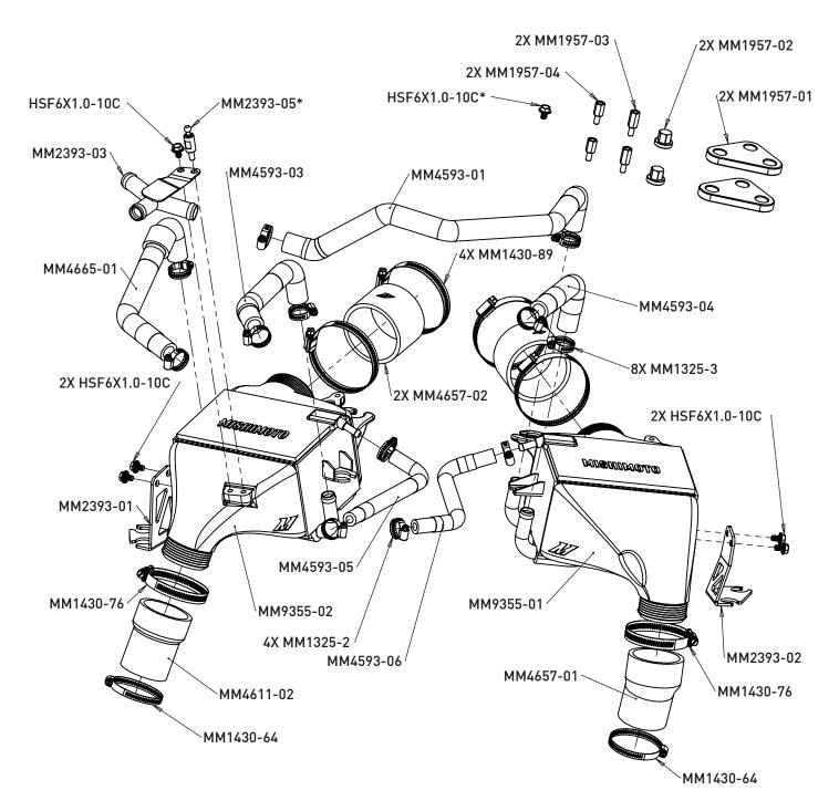
\*USE EXTRA HSFX1.0-10C BOLT IN PLACE OF MM2393-05 STAND OFF IF INSTALLED WITHOUT ENGINE COVER
