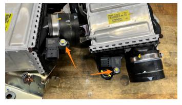
**15.** Remove the 8x rubber grommets from the stock intercooler brackets by pulling the metal collars out. The grommets can then be removed from the brackets. See photos on the following page.
