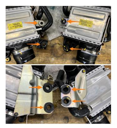
16. Install two of the grommets into each the Mishimoto intercoolers, ensuring that the flange side of the metal collars are facing up like they were in the stock intercoolers.
