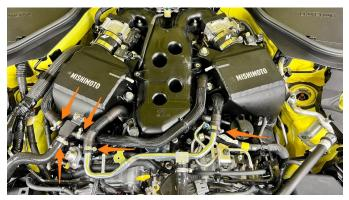
**27.** Install hoses 5 and 6 as shown and secure using 4x of the supplied 12-20mm worm gear clamps (7mm socket). Remove the stock engine cover mounting pegs (10mm socket).
