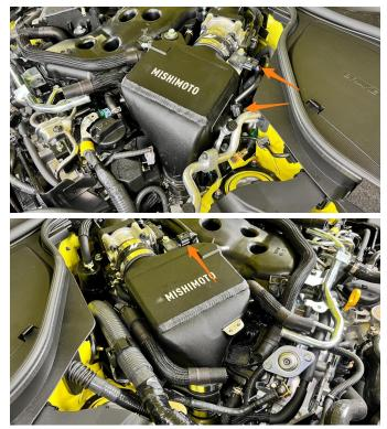
25. Install the Y-pipe onto the passenger side intercooler. Note:
