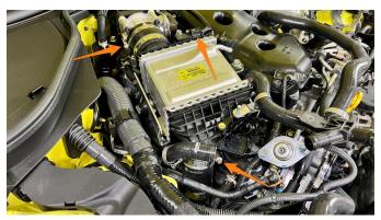
**9.** Using a 12mm socket, remove the 3x mounting bolts on the passenger side intercooler.
