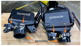
20. Slide a 40-64mm worm gear clamp over the small end of each of the turbo couplers then install them onto the turbo outlet. Drop a 52-76mm worm gear clamp onto each of the turbo couplers. Note: Ensure the clamps are oriented so you can access the tightening screw once the intercoolers are installed.
