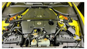
**5.** Use a 5mm Allen wrench to remove the 3x engine cover bolts and lift on the four corners to release it from the pegs. Remove the cover.
