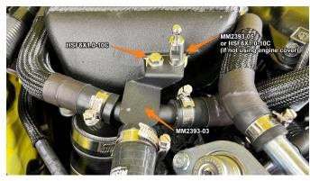
**26.** Slide a 16-25mm worm gear clamp over each of the 5x hoses
