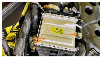
**10.** Using a 7mm socket, loosen the 2x intercooler hose clamps and unplug the 2x sensor connectors on the driver-side intercooler.
