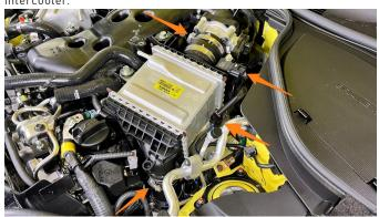
**11.** Using a 12mm socket, remove the 3x mounting bolts on the driver-side intercooler.
