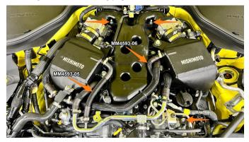
**28.** Install the provided mounting pegs/studs as shown.
