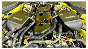
**29.** Reinstall the engine covers using the 3x stock bolts (5mm Allen wrench). Place one of the provided spacers on each strut tower where the bar mounts. Reinstall the strut bar on top of the spacers using the 4x stock bolts and the 2x provided nuts.
