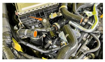
8. Using a 7mm socket, loosen the 2x intercooler coupler hose
