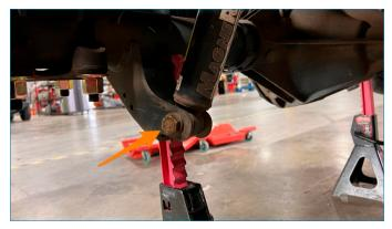
**08.** Using a 21mm deep socket, remove the 4 U-bolt nuts, U-bolts, and support bracket.
