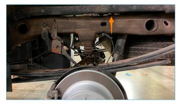
**06.** Using a 13mm socket, remove the bolt for the brake line bracket on top of the differential housing.
