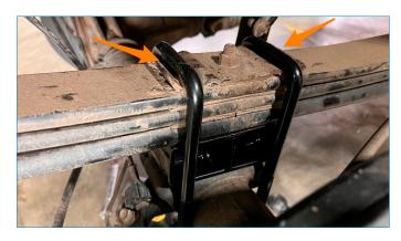
11. Using the supplied nuts and washers, install the lower support bracket and tighten using a 21mm deep socket to factory torque specifications.
