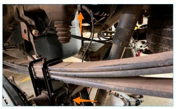
**04.** Using a 13mm socket, remove the bolt for the parking brake cable bracket on the driver's side and let the bracket hang free.
