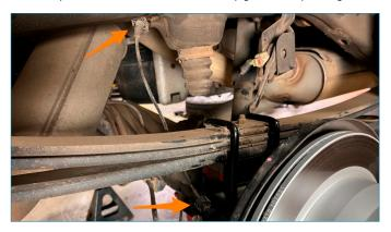
**03.** Use a pick tool to remove the ride height sensor pigtail on the driver's side.
