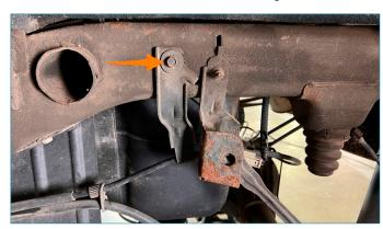
**05.** Using a 13mm wrench, remove the two bolts for the upper brake line bracket. These are on top of the frame rail on the driver's side.
