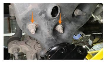
13. Remove the vacuum lines from the hub locker.
