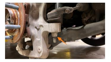
09. Using an 18mm wrench, remove the upper control arm ball joint nut. Counter-hold the threads using an 8mm socket. Loosely reinstall the nut so that the top of the nut is flush with the end of the threads. Using a hammer, hit the end of the threads to remove the tie rod end from the knuckle.
