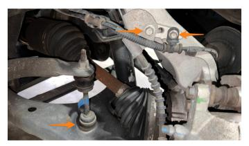
**04.** Using a 21mm socket, remove the two brake caliper carrier bolts. Remove the caliper assembly and secure it out of the way. Do not let it hang from the brake hose!
