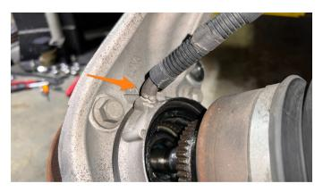
14. Let the jack down from the lower control arm. Push down on the lower control arm until the axle can be pulled from the hub. Hook the axle shaft on the sway bar end link threads to hold it out of the way. Be careful not to damage the wheel bearing seal in the hub when removing axle.
