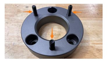
16. Install the spacer onto the top of the strut. It will only go on in one orientation. Using the supplied M10 washers and lock nuts, install the spacer onto the strut. Use a pry bar against the threads to keep the strut from rotating while tightening the nuts.
