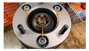
17. Reinstall the strut in the truck top-first, aligning the upper strut studs with the holes in the strut tower. Thread one of the upper strut nuts partially on to hold it in position.
