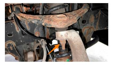
**07.** Hook the tie rod on the sway bar to keep out of the way. Remove the lower strut nut and bolt using a 21mm socket and 21mm wrench.
