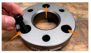
11. Fit the spacer onto the top of the strut. It will only go on in one orientation. Using a 17mm socket, install the spacer using the supplied M10 washers and lock nuts. Use a pry bar against the threads to keep the strut from rotating while tightening the nuts.
