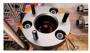
12. Reinstall the strut in the truck top-first, aligning the upper strut studs with the holes in the strut tower. Thread one of the upper strut nuts partially on to hold it in position.
