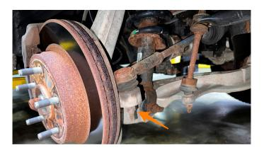
**06.** Using a 21mm wrench, remove the upper control arm ball joint nut. Counter-hold the threads using a 10mm socket. Loosely reinstall the nut so that the top of the nut is flush with the end of the threads. Using a hammer, hit the end of the threads to remove the tie rod end from the knuckle.
