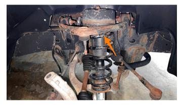
13. Pry down on the lower control arm until you can get the bottom of the strut over the front of the control arm and the bushing. Then, reinstall the lower strut nut and bolt.
