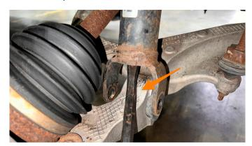
10. Install three of the supplied M10 socket head bolts into the threaded holes of the spacer until bottomed out and tighten using an 8mm Allen/hex key.
