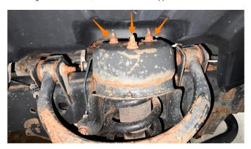
**09.** Using a pry bar, remove the strut by prying between the strut and the control arm. Pry down on the arm, up on the strut, and pull the strut outward toward you.
