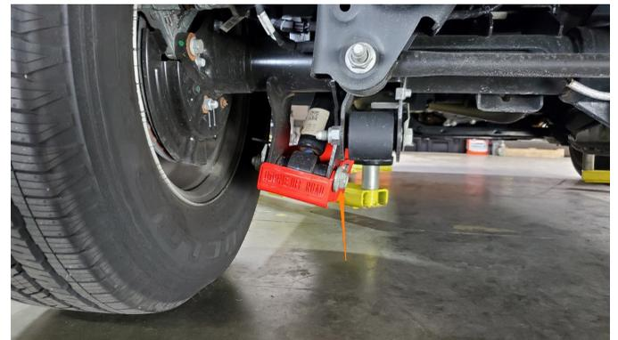
**NOTE:** If you do not have a torque wrench that reaches 350 lb-ft, tighten the bolt to 150 lb-ft and mark it as shown in the photo below. Then, tighten the bolt an additional half turn (180°).
