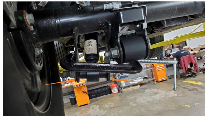
**02.** Using a 27mm socket loosen the driver side lower strut mounting bolt and remove the nut. A long breaker bar may be needed to get this bolt loose. The factory service manual recommends replacing this bolt and nut with a new bolt and nut when reinstalling.
