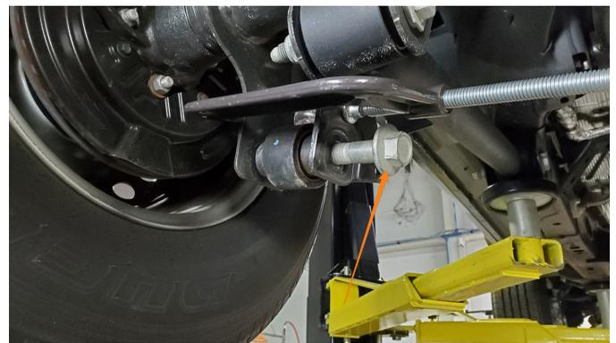
**03.** Install the skid plate onto the lower strut mount. The tab on the skid plate with the full hole will go onto the end of the strut mounting bolt as shown in the photo below. The "BORNE OFF-ROAD" logo faces the rear of the vehicle. (Image on next page)
