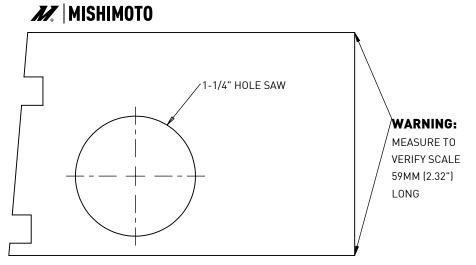
PLACE DRILLING TEMPLATE ON INSIDE OF TOW HOOK COVER
