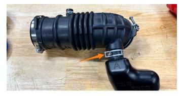
**3.** Slide the 30-45mm hose clamp onto the large port on the Mishimoto intake hose and install the resonator removed in the previous step in the orientation shown. Using a 7mm socket, tighten the hose clamp.
