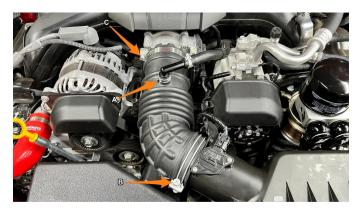
2. Using channellock or needle nose pliers, loosen the hose clamp and remove the plastic resonator from the stock intake hose.
