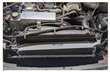
12. Using the Mishimoto supplied boot kit, attach the appropriate boots to their corresponding locations. Please note, of the two longer boots included with your kit, one boot is slightly larger internal diameter than the other. Use the larger diameter boot on the larger, passenger side outlet of the intercooler. Note the location of the bead inside the boot. This bead should go onto the intercooler pipe.
