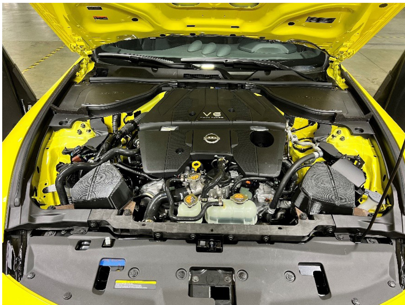
Figure 3: Mishimoto Intake in Closed Airbox Configuration (3D printed prototype)
