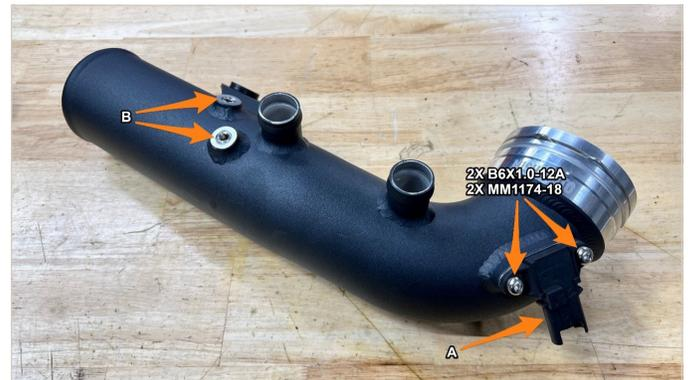
3. Install the 2x small straight couplers onto the pipe and use an 8mm socket to secure them with two 45mm worm gear clamps.
