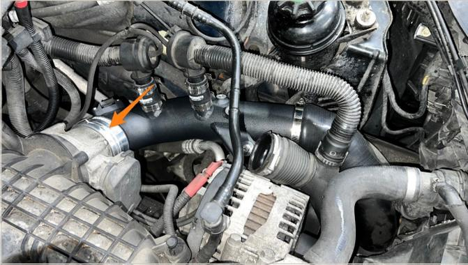
6. Rotate the angled coupler (A) until it lines up with the stock charge pipe (B), then push it on. Use an 8mm socket to tighten both worm gear clamps.
