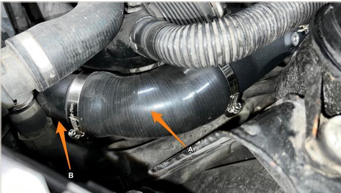
7. Using a 10mm socket, fasten the pipe bracket to the mount on the engine with the provided 6mm bolt. Slide two of the 45mm worm gear clamps onto the straight couplers, then push the stock recirculation valves into the couplers (B). Use an 8mm socket to tighten the worm gear clamps.
