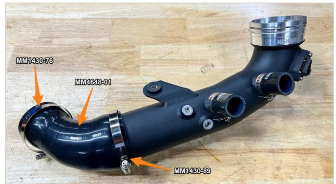
5. Install the charge pipe assembly into the vehicle throttle body side first. Push the pipe into the quick-disconnect fitting until you hear the clip snap into place.
