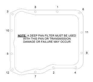
**05.** Refer to the factory service manual for proper transmission fluid fill procedures. The Mishimoto transmission pan adds approximately 6.1qt capacity. Be sure the proper fluid levels are reached before starting or driving the vehicle, or transmission damage could occur.
