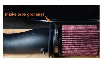
7. Slide the intake tube grommet over the intake tube, then install the air filter.[1x MM4545, 1x MM1672]
