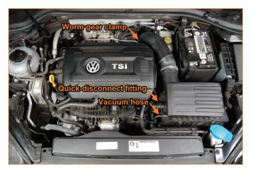
2. Remove the stock airbox and intake tube. (1x worm gear clamp, 1x vacuum hose, 1x quick-disconnect fitting)
