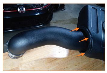
Install the intake tube assembly into the airbox. Starting from one spot, push the intake tube grommet into the airbox cutout until it is fully seated.
