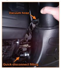
10. Place the intake assembly into the engine bay and connect the vacuum hose and quick-disconnect fitting.
