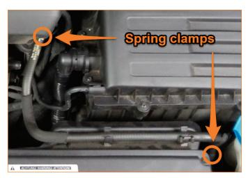
4. Remove the stock coolant hose from the driver's side of the radiator. (2x spring clamps)
