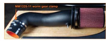
8. Install the coupler to the intake tube using the provided worm gear clamp. (1x MM1325-11)
