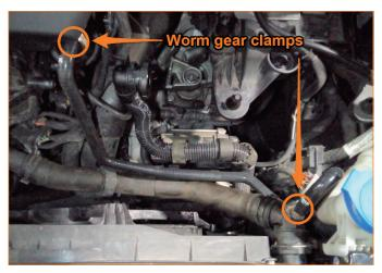
5. Install the Mishimoto coolant overflow hose using the provided clamps. (2x MM1325-2)
