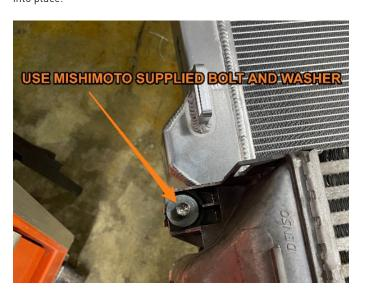
14. Reinstall the fan shroud. Use the included brackets included with the Mishimoto radiator using the 2x supplied M5 x 16mm bolts as shown. Repeat for the other side and remember to re-connect the electrical wire harness for the fan.
