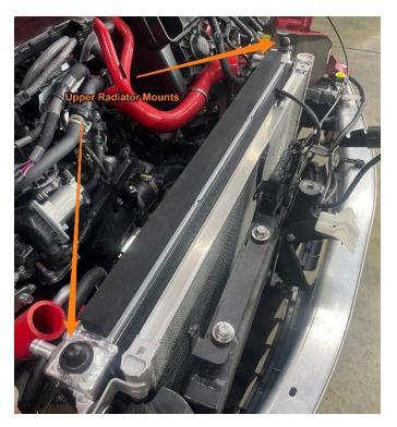
13. Re-install the intercooler. Use the Mishimoto supplied M6 x 30mm bolt and washer on the upper passenger side mount. Make sure the intercooler is fully seated in the lower peg mount. Use the factory bolts for the driver's side mounts. Torque the bolts to 6 Nm. Reconnect the rubber charge pipes and secure the hose clamps. Make sure all the radiator and intercooler shrouds are clipped back into place.
