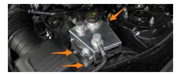
6. Install the coolant hoses onto the Mishimoto tank and secure them with the stock clamps. (Bottom hose not visible in photo)
