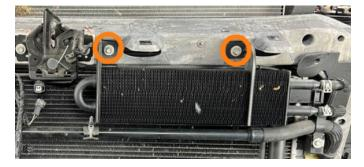
**65.** Place MM1666-01 and MM1666-02 onto each power steering cooler mount, as shown in the image below. Once done, secure the power steering cooler using the previously removed 10mm bolts. [2x MM1666-01 and 2x MM1666-02] [Image on next page]
