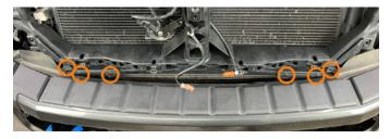
**55.** Remove the 10mm bolts securing the top of the grille support structure to the radiator support.
