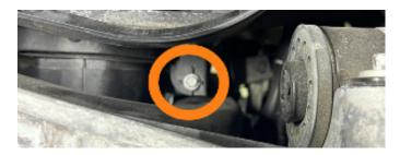
**51.** Unplug the horn wire harness connector, then unclip the wiring harness from the grille support structure.
