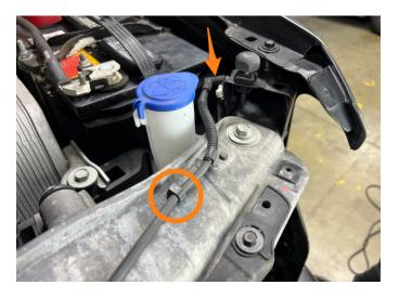
**54.** Remove the tree clips securing the lower radiator ducting to the grille support structure.
