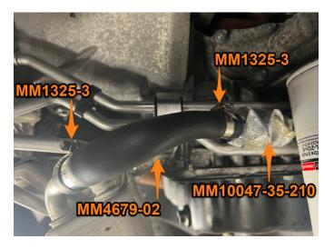
**31.** Carefully pull MM10047-35-210 over the hose and clamps installed in the previous step.
