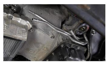
14. Place MM10013 over the two transmission lines at the front of the engine, then clamp MM10014 over the top of MM10013.(1x MM10013, 1x MM10014)
