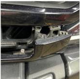
**41.** Remove the two 10mm bolts securing the grille to the bottom of the grille support structure.
