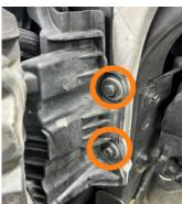
**57.** Remove the tree clips at the top outer corners of the grille support structure's inner ducts. Once the tree clips are removed, remove the grille support structure from the vehicle.
