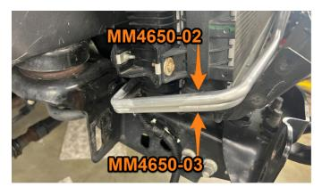
**70.** Connect MM4650-02 to MM1660 using MM4242-24 as shown in the image below. Secure in place using two of the provided worm gear clamps. Repeat this process for MM4650-03. [2x MM4242-24 and 4x MM1325-2]
