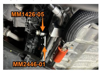
**16.** Fasten MM2446-01 to MM10014 using the provided M4 bolts. (4x BF4X0.7-10B)
