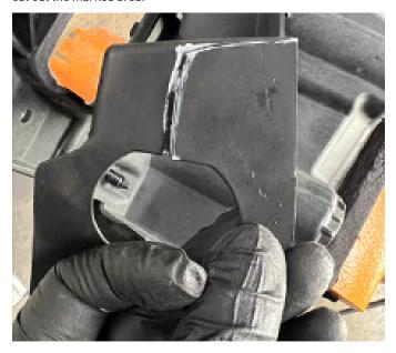
85. The image below shows how the driver-side grille support structure inner duct should look after being modified.
