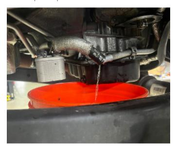
4. Remove the two clamps securing the coolant hose to the driverside coolant line on the stock liquid-to-liquid cooler. Partially remove the coolant hose from the line to allow any residual coolant left in the primary cooling system to drain in a controlled manner. Once drained, remove the hose from the stock liquid-to-liquid transmission cooler.
