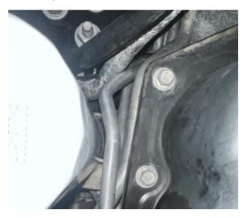
23. Confirm that the Mishimoto transmission lines are not contacting the oil pan, coolant line bracket, or other objects along their routing path.
