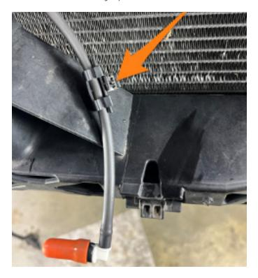
**88.** Reinstall the grille support structure. Check to make sure it is not rubbing on the Mishimoto transmission cooler or transmission cooler lines. (Image on top right)
