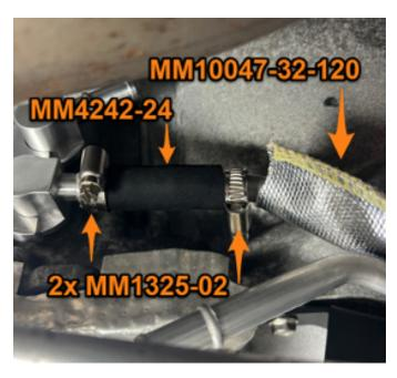
**33.** Attach one MM4242-24 to each end of MM4650-01 and secure it using two of the provided worm gear clamps. [1x MM4650-01, 2x MM4242-24, and 2x MM1325-2]
