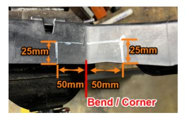
**80.** Mark the areas shown in the image belows on the passenger side of the grille support structure. Using an angle grinder, cut out the marked area.
