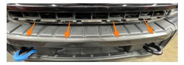
**44.** Disconnect the front camera and camera washer hose from the grille. Once disconnected, remove the grille from the vehicle.
