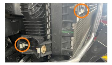
**72.** Install MM2446-03 onto the lower AC condenser mount using the previously removed bolt.
