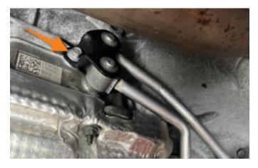
7. Remove the three bolts securing the stock transmission cooler to the bottom of the transmission. Once the bolts are removed, remove the stock transmission cooler from the transmission. Have a drain pan ready to catch any fluid spillage. (3x 13mm bolts)
