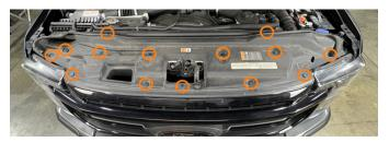
**39.** Remove the 10mm bolts securing the grille to the top of the grille support structure.
