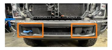
**62.** Remove the 15mm bolts securing the inner bumper brackets to the chassis on both sides of the vehicle.
