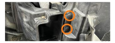
49. Remove the upper air intake duct from the air box.
