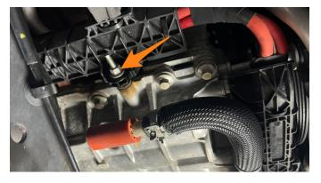
9. Remove the nut securing the coolant line and rear section of the battery wire harness to the passenger side of the engine. Once the nut is removed, remove the coolant line bracket from the stud.
