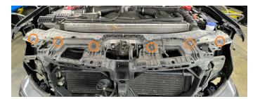
**56.** Remove the 13mm bolts securing the sides of the grille support structure to the radiator support. (Images on top right)
