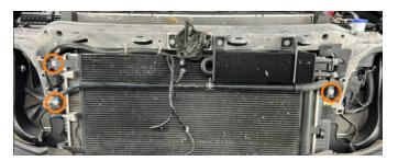
**67.** Loosely install MM1664-02 onto the passenger side of the secondary radiator, as shown in the image below, using two of the provided M6 bolts. Loosely install MM1664-01 onto the driver side of the secondary radiator, as shown in the image below. Fasten MM1660 between MM1664-01 and MM1664-02 using the provided M6 bolts. Tighten all the bolts. (1x MM1660, 1x MM1664-01, 1x MM1664-02, 3x HF6X1.0-20A, and 4x HF6X1.0-14)
