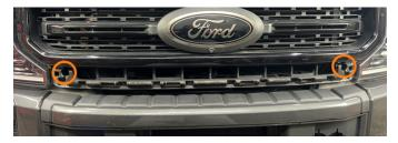
**42.** Remove the two 10mm nuts securing the grille to the top of the grille support structure.
