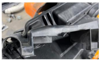
84. Mark the area shown in the image below onto the driver-side grille support structure inner duct. Using a razor knife or scissors, cut out the marked area.
