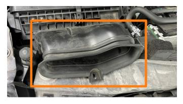
**50.** Remove the 8mm fastener securing the lower air intake duct to the air box and then remove the duct from the vehicle.
