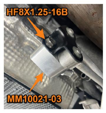
**29.** Reinstall the transmission pan heat shield, then install MM2446-05 to both the transmission and MM10021-03. Torque all fasteners to 80 lb.in (9Nm).
