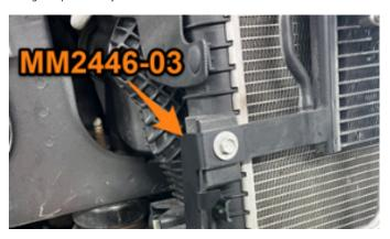
73. Place MM10013 over the two transmission lines at the side of the secondary radiator, then clamp MM10014 over the top of MM10013. Secure MM10014 to MM2446-03 using the provided M4 bolts. [1x MM10013, 1x MM10014, and 4x BF4X0.7-10B]
