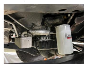
3. Remove the two clamps securing the coolant hose to the passenger-side coolant line on the stock liquid-to-liquid transmission cooler. Partially remove the coolant hose from the line to allow any residual coolant left in the primary cooling system to drain in a controlled manner. Once drained, remove the hose from the stock liquid-to-liquid transmission cooler.
