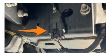
**59.** Unclip the block heater wire harness from the back side of the bumper (passenger side of the vehicle). (Image on next page)
