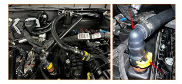
**08.** Attach CCV-side catch can hoses as shown and secure with provided worm gear clamps.
