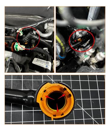
**03.** Remove the plastic caps and expose the two M6 studs for mounting the catch can bracket.
