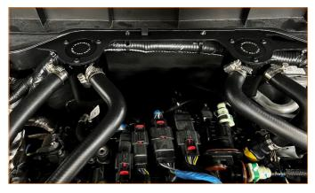
**07.** Attach PCV-side catch can hoses as shown and secure with provided worm gear clamps. Push down on the fittings to engage the barb, then push in the yellow locking tab.
