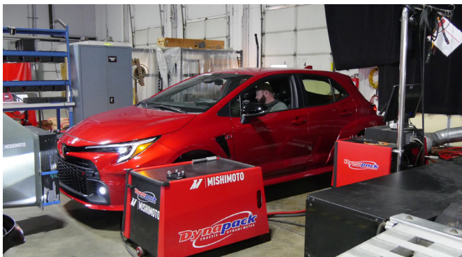
Figure 6: A Dynapack dynamometer was used for vehicle testing.
