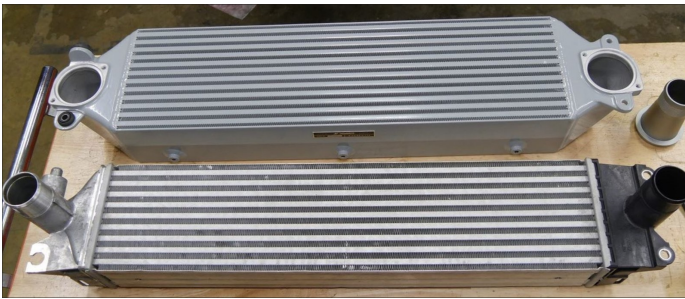
Figure 3: Comparison of the stock intercooler to the Mishimoto intercooler.
