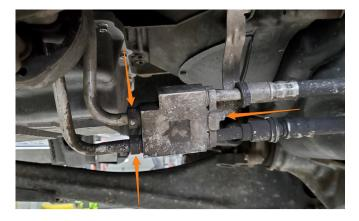
**3.** Replace the stock o-ring on each of the two (2) transmission-side lines with the two (2) supplied new o-rings. Then, replace the stock dowty seal on each of the two (2) cooler-side lines with the two (2) supplied new dowty seals.
