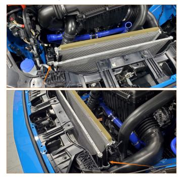
9. Steps 9-14 only apply to 2.3L vehicles. For V8 vehicles, skip to Step 15. Using a 10mm socket, remove the six (6) bolts on the top of the bumper.
