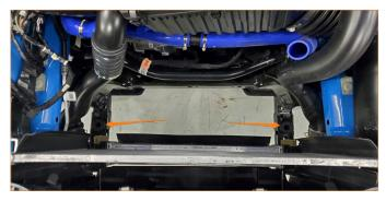
**16.** Lower the Mishimoto radiator into the vehicle and insert the lower mounting pegs into the rubber grommets.
