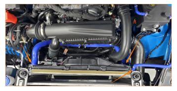
**5.** Disengage the red locking tab on the fan plug and disengage the plug. Then, remove the tree clips from the fan shroud to separate the wiring harness from the shroud.
