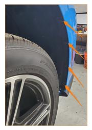
11. Pull back the wheel liner to access the tree clip in the upper corner of the bumper and, using a flathead screwdriver, remove the tree clip from both sides of the vehicle. Using a 10mm socket, remove the two(2) bolts inside the fender that secure the bumper to the vehicle on both sides of the vehicle.
