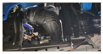
Using pop clip pliers or a flathead screwdriver, remove the eight (8) pop clips from the radiator cover and remove the cover from the vehicle.
