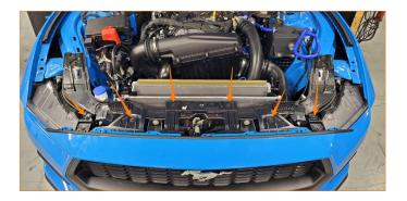
10. Using pop clip pliers or a flathead screwdriver, remove the four(4) pop clips securing the wheel liner to the bumper on each side of the vehicle.
