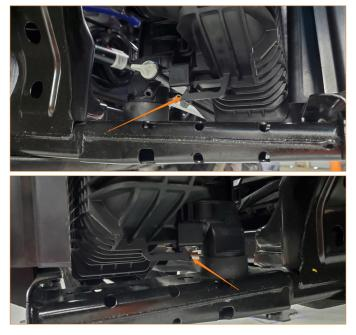
**15**. Remove the radiator from the vehicle by lifting it straight up. If the rubber grommets remained attached to the lower mounting pegs on the radiator, remove them and reinstall them into the vehicle's frame.
