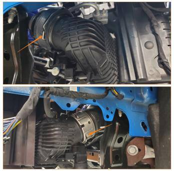
**14.** Disengage the plastic clips securing the bottom of the intercooler from the radiator and tilt the bottom of the intercooler away from the radiator. Then, lift the intercooler upwards to separate the upper intercooler mounts from the hooks on the radiator.
