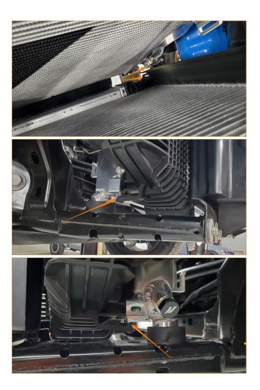
**18.** Place the tabs on the A/C condenser into the hooks on the radiator. Then, using a 10mm socket, secure the A/C condenser to the radiator with one (1) of the supplied M6 washers and bolts.
