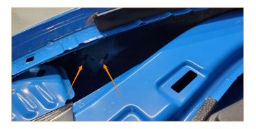
12. Unplug any wiring connections on the inside of the bumper (connections may vary depending on vehicle trim level and options).Then, remove the bumper from the vehicle.
