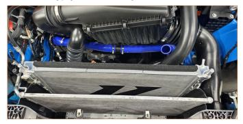
**17.** This step only applies to 2.3L vehicles. For V8 vehicles, skip to Step 18. Attach the upper mounts on the intercooler onto the hooks on the radiator. Then, push the lower intercooler mounts into the mounts on the radiator to engage the plastic clips.
