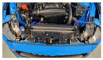
**25.** Attach the wheel liner to the bumper on both sides of the vehicle with the eight (8) pop clips that were removed in Step 10.
