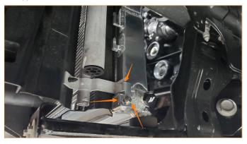
**27.** Using a 7mm socket, reinstall the engine splash guard using the twenty (20) bolts and three (3) pop clips that were removed in Step 1.
