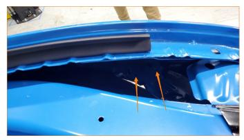
**24.** Using a 10mm socket, reinstall the six (6) bolts that were removed from the bumper in Step 9.
