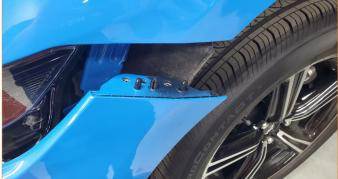
23. Using a 10mm socket, reinstall the four (4) bolts that were removed in Step 11 – two (2) on each side of the vehicle.
