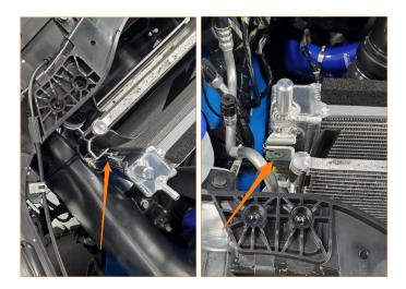
**19.** Reinstall the stock fan shroud by inserting the tabs on the bottom of the fan shroud into the hooks on the back of the radiator. Then, reinstall the stock radiator mounts onto the upper mounting pegs on the Mishimoto radiator and, using a 10mm socket, secure them with the four (4) bolts that were removed in Step 7.
