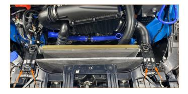
8. Using a 10mm wrench, remove the one (1) bolt securing the A/C condenser to the radiator. Then, disengage the plastic clip securing the tab on the other side of the A/C condenser and lift the condenser straight up to separate the tabs on the condenser from the hooks on the radiator. Depending on the vehicle trim level and options, additional coolers may be present. If so, separate them from the radiator the same way as the A/C condenser.
