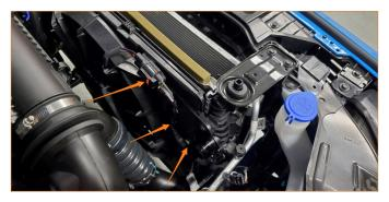
6. Using a 10mm socket, remove the two (2) bolts securing the fan shroud to the radiator.
