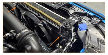
7. Using a 10mm socket, remove the two (2) bolts from each of the upper radiator mounting brackets and remove the brackets from the vehicle.
