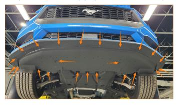
**28.** Reinstall the radiator cover using the eight (8) pop clips that were removed in Step 3.
