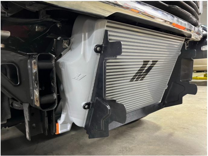
Figure 3: Mishimoto Intake Production Sample Installed
