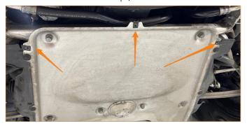
**5.** Remove 6x screw clips from the factory oil cooler skid plate and install them in the locations shown.
