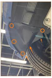
**3.** Remove the 7x 8mm screws and 2x 13mm bolts holding the factory oil cooler skid plate to the vehicle and remove the skid plate from the vehicle.
