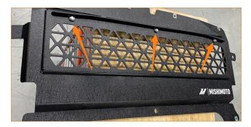
7. Install the weather stripping onto the diffuser as shown, making sure that the weather stripping is centered on the diffuser. It may be necessary to push down on the weather stripping with force for it to be fully seated. Alternatively, use a flathead screwdriver to open up the channel in the weather stripping for an easier installation. If a screwdriver is used to open up the channel, use pliers or similar to clamp the weatherstripping onto the diffuser afterward.
