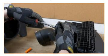
15. Insert the rubber grommets into the Mishimoto airbox.
