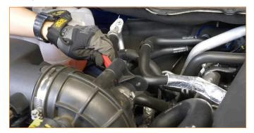
**07.** Loosen the clamps on either end of the intake tube. (2x worm gear clamps)
