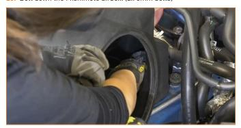
24. Bolt down the Mishimoto intake duct. (2x 8mm bolts)
