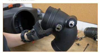
14. Remove the two inserts and grommets from the stock airbox.
