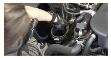
28. Slide the intake filter in first, and then rotate it to align with the coupler.
