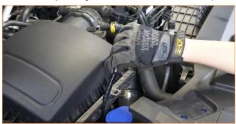
05. Separate the quick-disconnect by pulling the yellow tab out.
