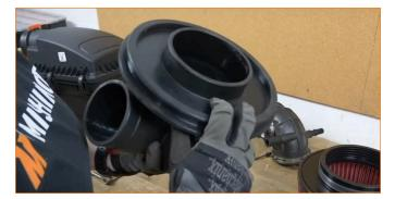
26. Slide the air filter over the intake tube. (1x worm gear clamp)
