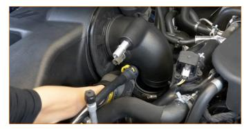
29. Once aligned, push the rubber grommet into place.
