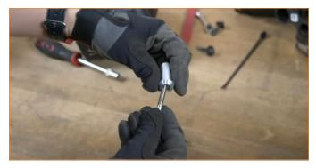
Install the assembled peg into the Mishimoto airbox. (5mm Allen key)
