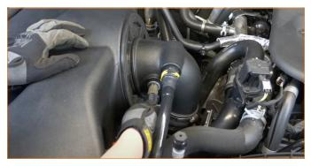
**33.** Wrap and secure the provided zip tie around the blow-off valve hose. Now attach this zip tie to the tree-clip zip tie that is already mounted on the coolant hose. The tree clip on the stock zip tie will push into the hole on the provided zip tie.
