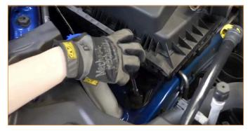
Lift the airbox and push toward the engine to disengage the rubber grommet.
