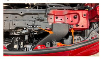
**8.** On the backside of the shroud, the cut line is marked in silver. The cut will be made on the inside of the reinforcing ribs, so they are retained for
