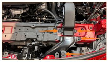
**7.** Install the Mishimoto air duct as shown and fasten using the stock pop clips.
