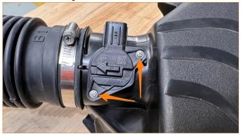
**14.** Install the MAF sensor into the Mishimoto MAF housing using the provided M4 hardware.
