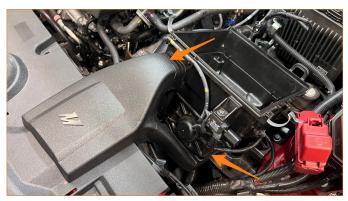
**13.** Remove the 2x screws (Phillips head) then remove the MAF senor from the stock housing.
