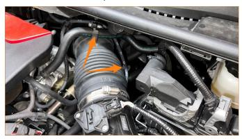
**3.** Release the two airbox clips and unplug the MAF sensor electrical connector. Remove the airbox lid and hose from the vehicle.
