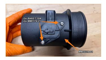
15. Insert the MAF housing into the Mishimoto airbox (flanged side first) then, install the air filter onto the MAF housing. Tighten the air filter hose clamp (8mm socket).
