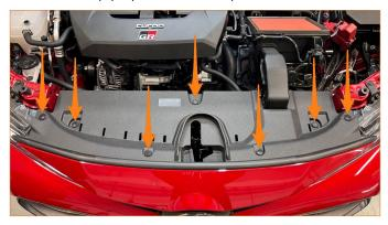
6. Remove the 4x pop clips then remove the two plastic intake ducts.
