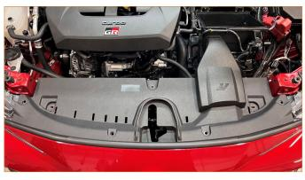
12. Ensure the top part of the snorkel is fully inserted into the inlet on the stock airbox and the bottom part of the snorkel is lined up with the lower inlet on the stock airbox. Secure the shroud with the stock pop clips.
