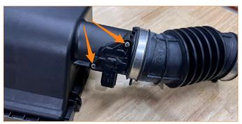
7. Install the MAF sensor into the Mishimoto MAF housing as shown using the supplied M4 hardware and tighten the screws (2.5mm hex key).
