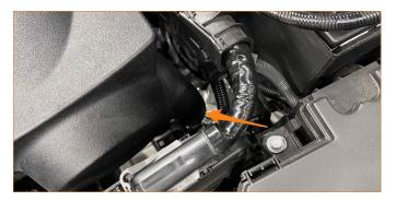
**11.** Install the MAF housing, filter, and grommet assembly into the airbox as shown, making sure the airbox is seated in the groove on the grommet all the way around the perimeter.
