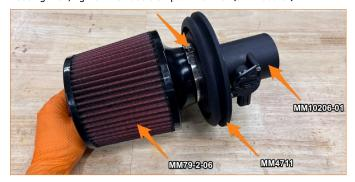
Install the Mishimoto airbox into the vehicle as shown and fasten using the 2x bolts (10mm) removed in step 4.
