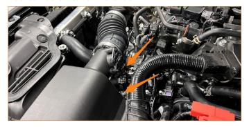
**3.** Remove the 4x bolts (10mm socket) and pop clip then, remove the lower half of the airbox from the vehicle.
