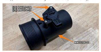
8. Install the grommet onto the MAF housing as shown, followed by the filter. Ensure they are pushed all the way up against the flange on the MAF housing then, tighten the hose clamp on the filter (8mm socket).
