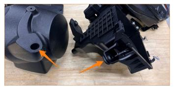
**6.** Remove the 2 screws (Phillips screwdriver) fastening the MAF sensor to the stock airbox lid then remove the MAF sensor from the housing.
