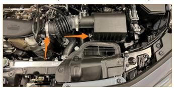
2. Unplug the electrical connector for the MAF sensor. Release the other airbox clip. Pull the loose end of the hose off the intake pipe then, remove the airbox lid and hose from the vehicle.
