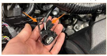
**13.** Plug the MAF sensor connector back in then, install the coupler as shown and fasten using the 2x supplied worm gear clamps (7mm socket).
