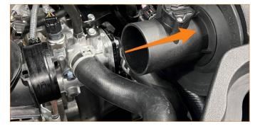
12. Remove the 90-degree outer housing from the MAF sensor plug.
