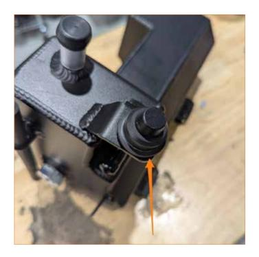
**4.** Transfer the hose from the stock tank onto the Mishimoto tank and secure it with the smaller of the two (2) provided worm gear clamps.
