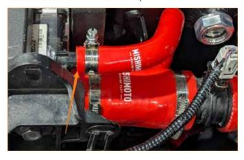
**7.** Secure the hose to the bracket on the tank with the supplied tree clip zip tie.
