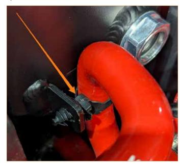
**8.** Connect the stock radiator hose to the lower port on the tank and secure it with the remaining supplied worm gear clamp.
