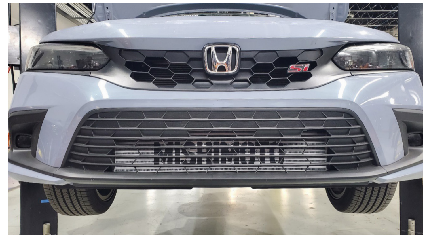
Figure 15: Mishimoto intercooler installed on the 2024 Honda Civic Si.
