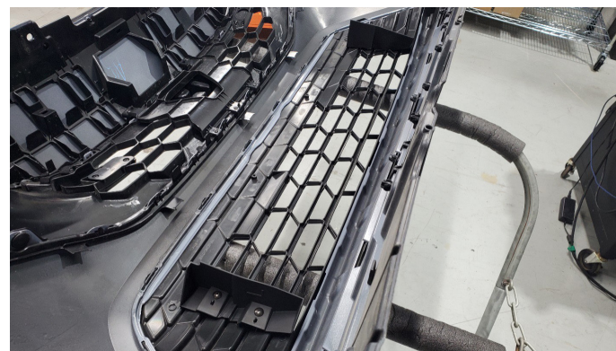
Figure 5: Mishimoto intercooler ducting installed on the Civic Si bumper.
