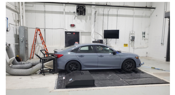
Figure 7: The 2024 Honda Civic Si being set up on the Mustang dynamometer and prepared for testing.
