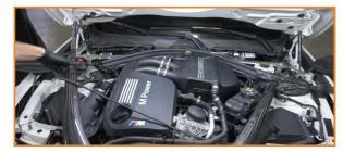
Lift the cover off the engine.
