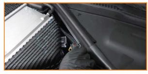
3. Loosen all the clamps on the intercooler pipes. (5x worm gear clamps)
