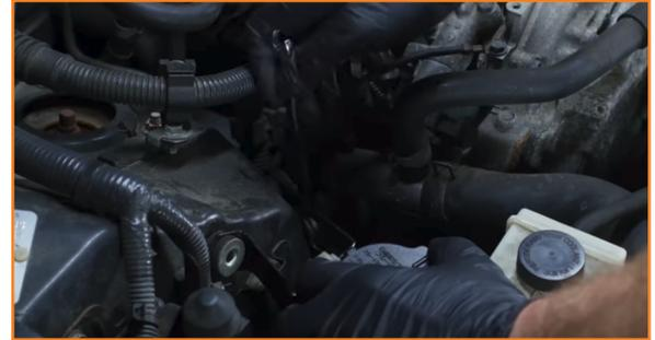
2. Slide the clamps down the hose connected to the PCV system. This will allow you to separate the hose from the valve cover and intake manifold ports. (2x spring clamps)
