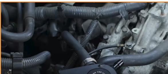
9. Install the larger hose to the intake manifold and OUT port on the catch can. Run this hose under the electrical harness near the engine port. (1x 12-20mm worm gear clamp, 1x 16-25mm clamp)
