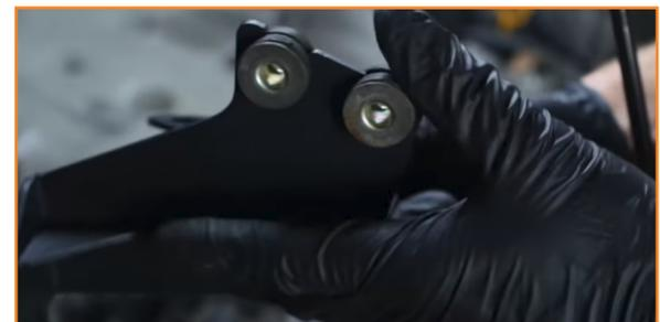
4. Install the Mishimoto catch can bracket using the original hardware from the stock bracket. Make sure to attach the power steering fluid container to the available slot on the Mishimoto bracket. (2x 10mm bolts)
