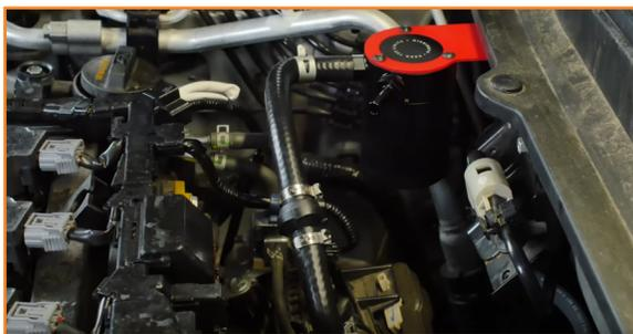
11. Install the inlet hose to the PCV valve and IN port on the catch can. (2x spring clamps)
