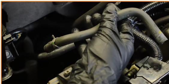
2. Remove the bolts on the fuel line cover. (2x 10mm bolts)
