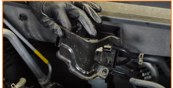
3. Remove the bolts that secure the fuel line bracket. (2x 10mm bolts)
