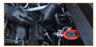
10. Reinstall the engine cover. Be sure to engage all four pegs.
