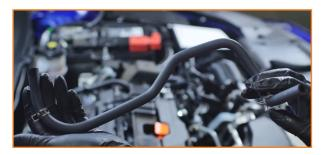
3. Remove the top bolts that secure the fuel line connector bracket to the firewall. (2x 10mm bolts)
