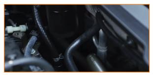
9. Install the check-valve hose. One end attaches to the catch can IN port. The other end goes to the port on the intake manifold at the back of the engine. (2x spring clamps)
