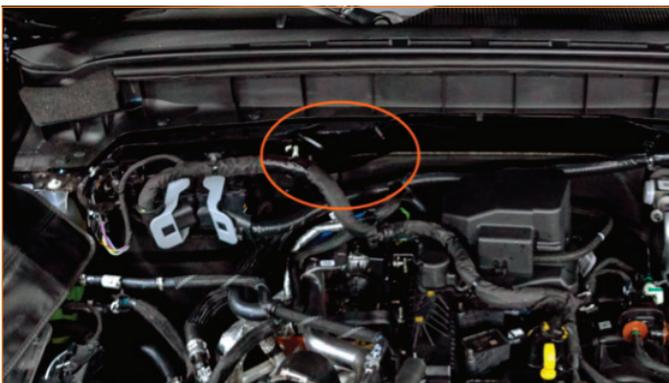
**02.** Remove one 10mm nut and cut the zip tie holding the wiring harness.
