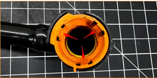
**03.** Remove the plastic caps and expose the two M6 studs for mounting the catch can bracket.
