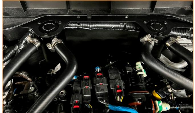
**07.** Attach PCV-side catch can hoses as shown and secure with provided worm gear clamps. Push down on the fittings to engage the barb, then push in the yellow locking tab.
