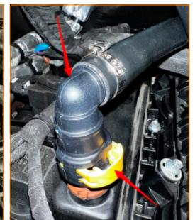
**08.** Attach CCV-side catch can hoses as shown and secure with provided worm gear clamps.
