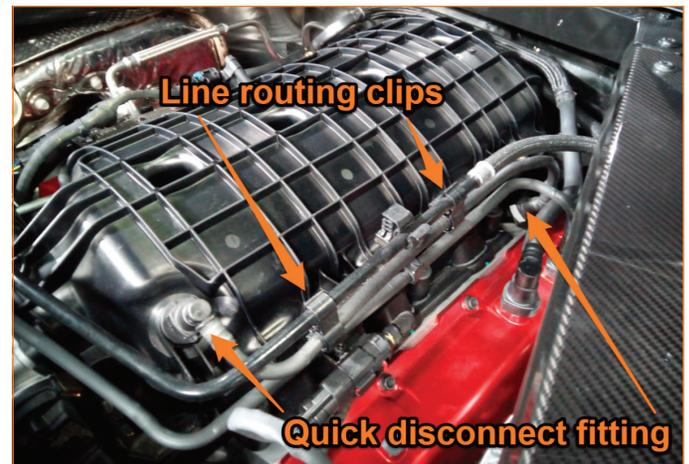
**02.** Install MM4553-03 hose to the PCV valve port. (1x MM4553-03 hose)
