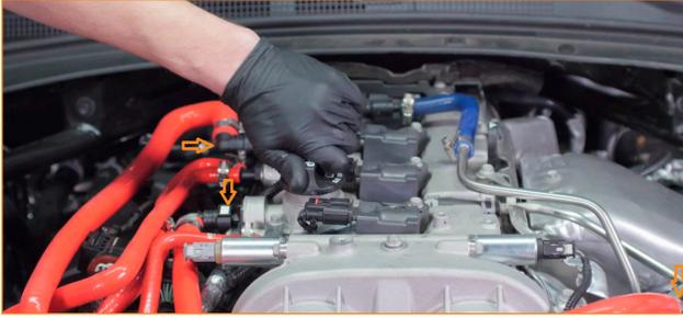
25. Turn the can until the lines flow smoothly and then tighten the two bolts that secure it to the bracket.
