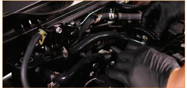
15. Now go back and fully tighten the Allen bolts that secure the catch can to the mounting bracket.
