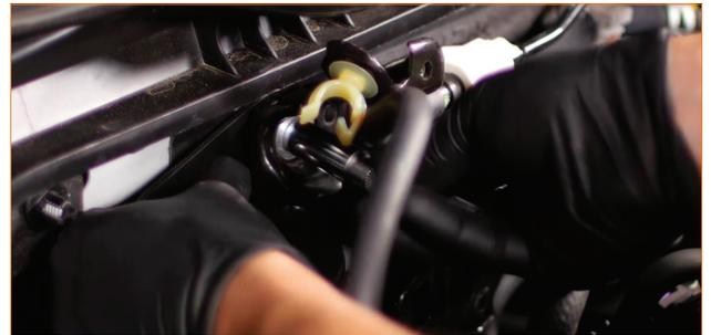
09. Move the fuel line back into place, and secure it with the white and black clips.
