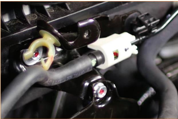
06. Move the fuel line out of the way to expose the mounting bolts.
