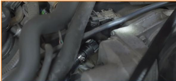
8. Install the catch can to the bracket.
