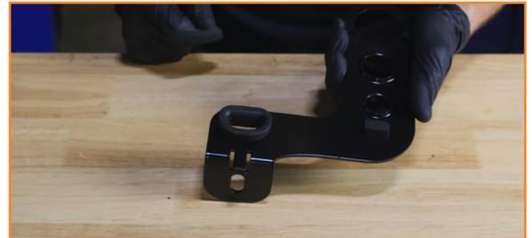
3. Slide the bracket onto the radiator. Secure the Mishimoto bracket where the upper radiator support used to be. (1x 10mm bolt)
