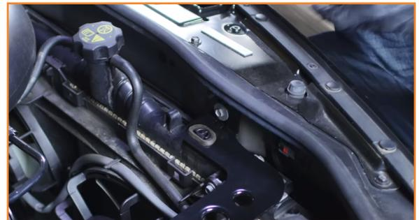
4. Remove the oil fill cap and remove the engine cover. Replace the oil fill cap before continuing.
