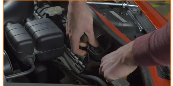
2. Transfer the bushing on the upper radiator support to the catch can bracket.
