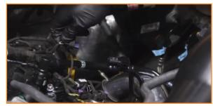
4. Separate the quick-disconnects on the CCV hose and remove it.
