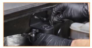
15. Attach the straight hose quick-disconnect to the CCV port on the engine.
