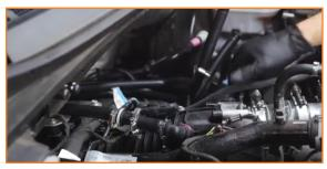
11. Attach the hose without a check-valve to the IN port on your catch can. (1x worm gear clamp)
