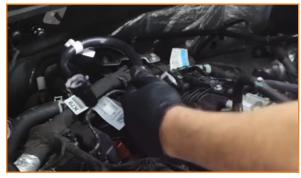
3. Disconnect the CCV hose's pressure sensor.
