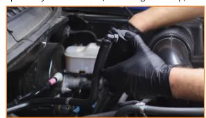
12. Attach the hose with a check-valve to the OUT port on your catch can. (1x worm gear clamp)
