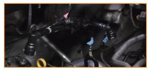
5. Pull the grounding strap harness off the bolt. Then remove the nut on that bolt. (1x 10mm nut)
