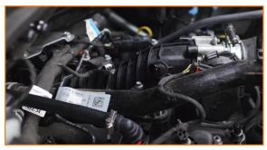
10. Install the hose with a check-valve to the OUT port on the valve cover.
