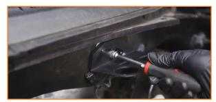
14. Install the catch can to the bracket. (2x 2.5mm screws)
