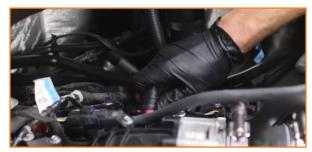
16. Install the hose with the pressure sensor to the intake port.
