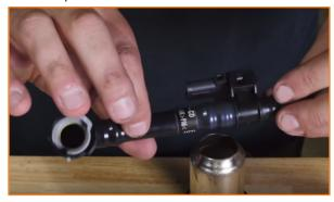
8. Transfer the pressure sensor to the provided hosing. The end without the electrical connector slides into the hose hose with the quick-disconnect. (2x worm gear clamps)
