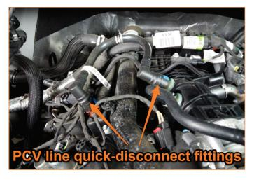
**02.** Remove the stock CCV line from the vehicle. (2x quick-disconnect fittings, 1x electrical connector)
