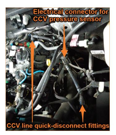
**03.** Using a heat gun, remove the CCV pressure sensor from the stock CCV line.
