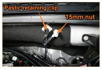
**12.** Secure the MM2227 bracket to firewall using the ground cable 15mm nut and the provided 10mm locking nut. (1x MM1163-10 locking nut)
