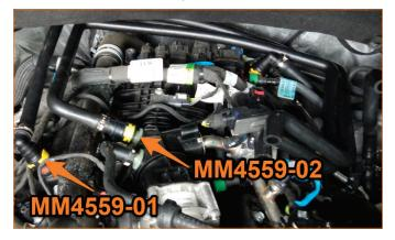
09. Connect MM4559-01 to the inlet port of the catch can.
