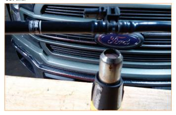
**04.** Connect the stock CCV pressure sensor to MM4559-04 and MM4559-05 as shown in the above image using the provided clamps. (2x MM1325-3 worm gear clamps)
