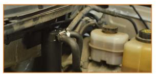
21. Reinstall the engine cover and oil cap. To properly reinstall the cover, slide the back end in first with the front end still raised. Then lower the front.
