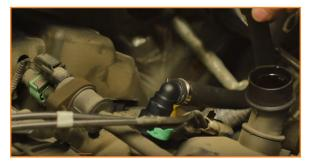
20. Attach the open end to the catch can's IN port. (1x worm gear clamp)
