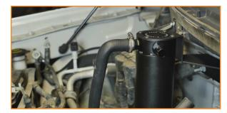
Connect the hose from the valve cover to the catch can's IN port. Secure the connection with one of the provided clamps.
