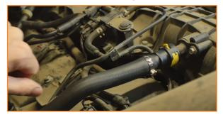
7. Connect the hose without a check valve to the valve cover. Again, the quick-disconnect end is what attaches to this port.
