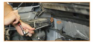
4. Secure the bracket overtop the ground and ECU cover. Align the holes on the bracket with the empty bolt holes on the ground and ECU cover. An extra bolt and nut are in your kit to hold the top of the bracket.
