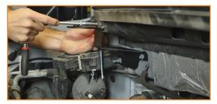
5. Disconnect both ends of the stock PCV hose and remove it.
