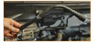
6. Connect your hose with the check valve to the intake manifold. The quick-disconnect end will be the side that attaches to this port.
