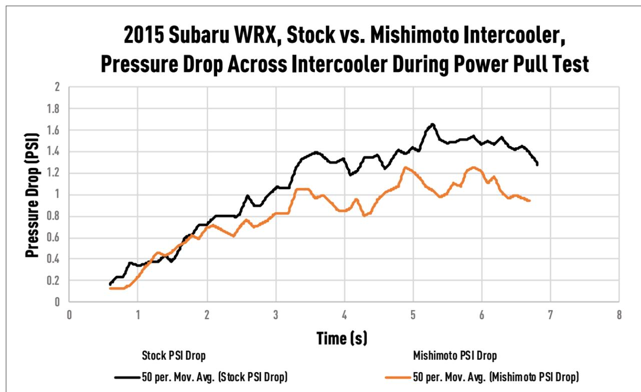
**FIGURE 6:** Stock intercooler pressure drop across the core. At the end of the run the stock core is at a 1.5 psi drop, and the Mishimoto core is at about a 1.2 psi drop.
