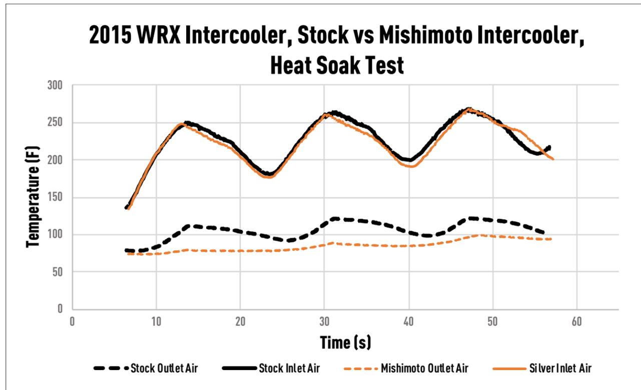
**FIGURE 5:** Mishimoto Intercooler Heat-Soak Test, notice how the stock intercooler temperatures are higher and rise faster than the Mishimoto core.
