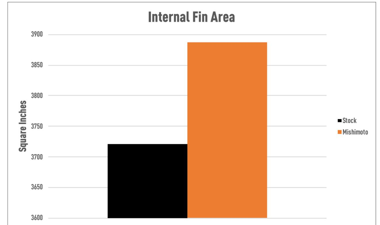
**FIGURE 2:** By reducing fin height and pitch, the surface area was increased by 27% compared to the stock core.
