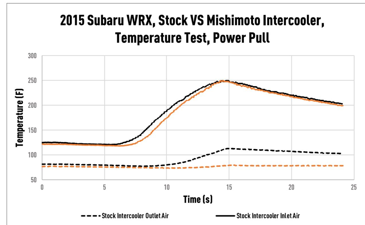
FIGURE 4: This is the chosen Mishimoto Intercooler vs the Stock Intercooler. Notice how the stock outlet rises during the dyno pull while the Mishimoto intercooler stays much flatter.
