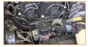
Lift the vacuum pump slightly so that you have enough room to slide the catch can brack under the pump. Align the holes in the bracket with the pump's grommets. With the bracket set, secure the bump using the original hardware. (2x 10mm bolts)
