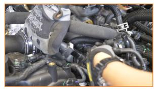
6. Separate the intake air temp sensor wiring from the intake pipe. Next, disconnect the sensor electrical harness from the intake.
