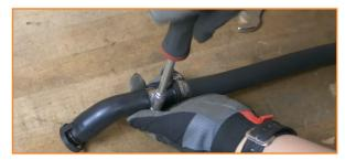
14. Route the hose with the rubber elbow under the bypass valve pipe and connect it to the valve cover. Route the other end under the turbocharger muffler and connect it to the IN port on the catch can. (1x worm gear clamp)
