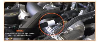
5. Squeeze the quick-disconnect fittings at each end of the crancase breather hose, and then remove the hose.
