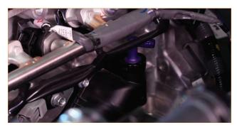
3. Reach around the back of the intake manifold (the firewall side) and locate the PCV hose where it attaches to the purple nipple on the PCV vent assembly (on the side of the engine block). The PCV hose is a short, U-shaped hose with no clamps.
